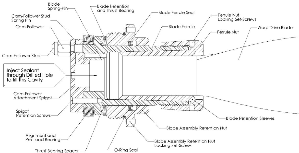
**Figure 2 - Cross-Section of Blade Assembly
